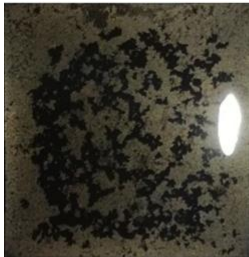
Figure 3 - Graphene agglomeration attains after the drop-casting method on a polished surface.
