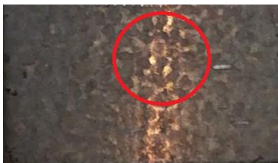
Figure 4 - GO coating defect exhibited on the polished surface.
